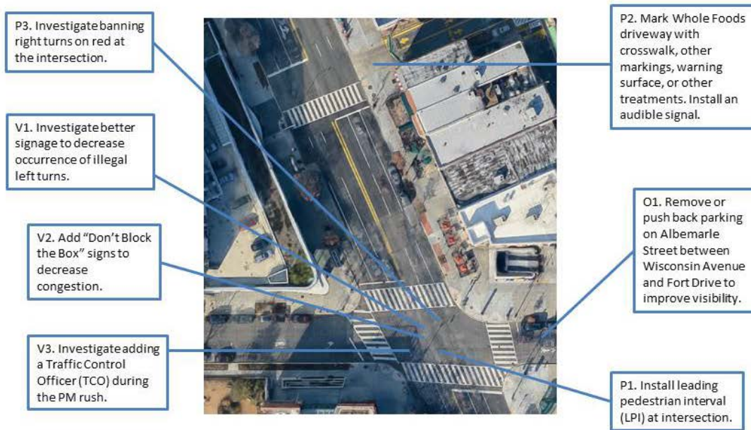
Figure 25. Wisconsin Avenue and Albemarle Street NW Site Visit Observations
