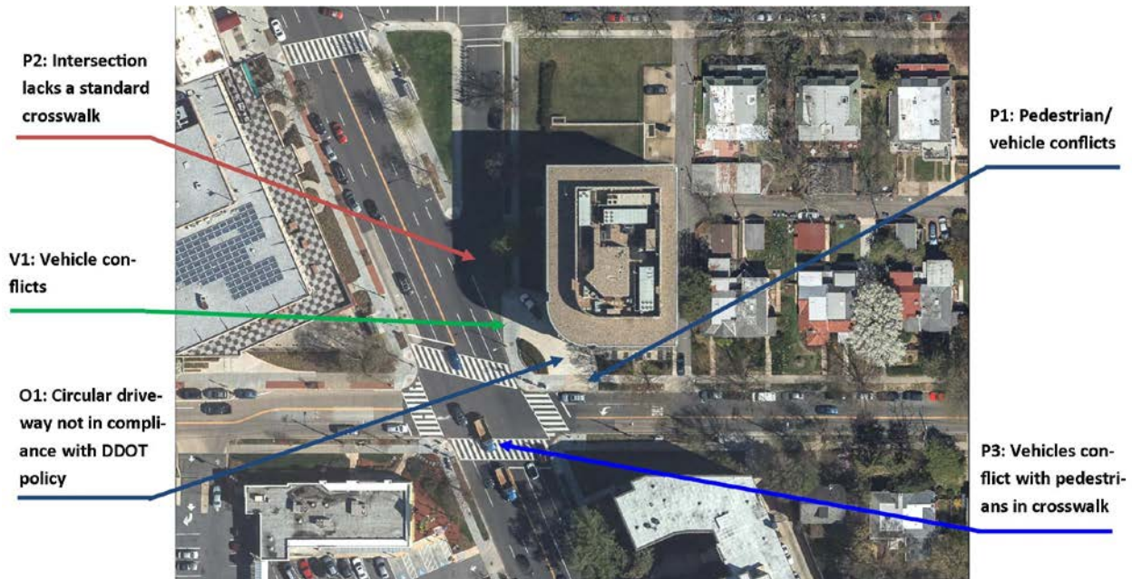
Figure 31. Wisconsin Avenue, Van Ness Street, and 39th Street NW Site Visit Observations
