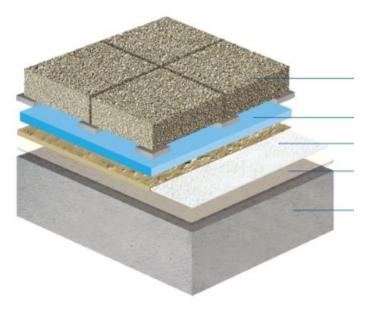
**The second** system is a 90 mil PVC installed over a durock over polyisocianurate insulation. This system is a membrane roof system that is fully adhered to the concrete deck with welded seams. This roof system is not as expensive as the IRMA roof but will function well over its lifespan. A budget number for this system is between \$25 and \$30 / sqft
